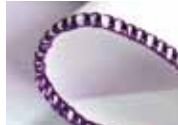
2-thread rolled edge Edge finish for lightweight fabrics. Nice finish on silky scarves, pillow ruffles and napkins.
